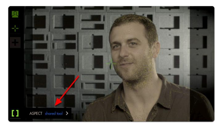
By default the Aspect Guide is set up for a 4x3 aspect ratio for times when you're needing to preview the cutoff area of an old-school monitor.
