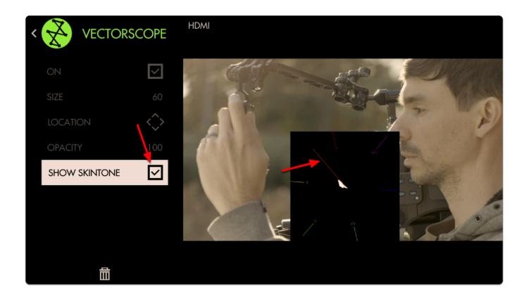
Because the **entire image** is being plotted to the graph all at once, we can check the status of individual areas by using **Pixel Zoom** in combination with the **Vectorscope** for **spot meter** functionality!
