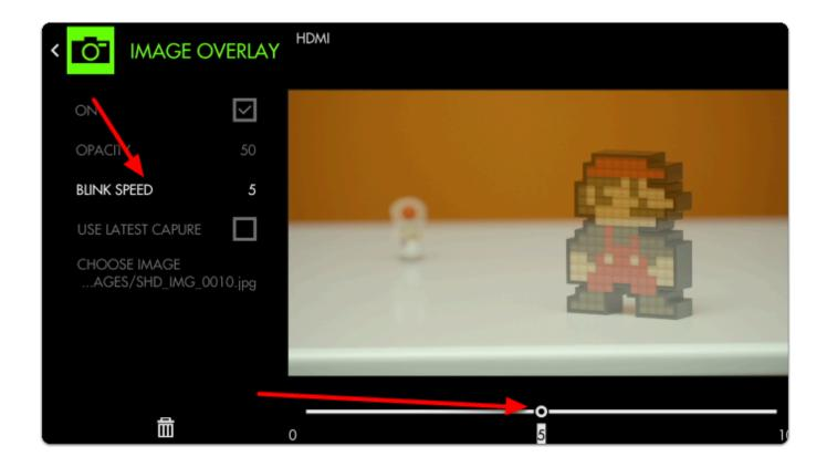
Increasing the **OPACITY** gives us a clearer distinction between the two images when blinking (if not set to blink, this will make the overlaid image completely opaque, covering the underlying feed)
