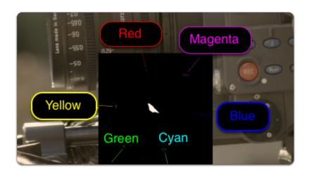
If we **apply a LUT** to this page, the Vectorscope reacts by **expanding** its plotted area. The scope confirms that we are viewing a more heavily saturated image after applying the look.
