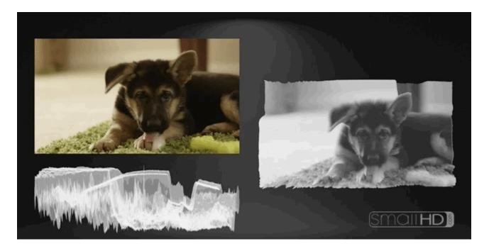
The **Waveform** is generally considered the **most robust exposure tool** because it plots your image's luminance (brightness) -- and chrominance if using <u>RGB mode</u> -- to a graph but unlike the Histogram, it physically **matches the screen from left-to-right**.
