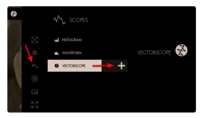
A **Vectorscope** appears at the bottom of the image. The **'blob'** is largely contained in the **center** of the graticule/crosshairs which means the colors of the current image are **not very saturated** (which is especially true as this footage is using log-based gamma).
