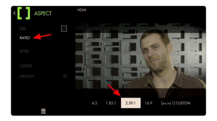
Navigate to "Ratio", select it and change the aspect ratio to "2.39" for cinemascope viewing.
