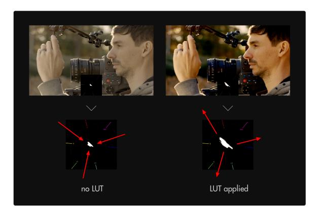
The Vectorscope uses the same layout as a **color wheel** and therefore principles of **color** theory apply - for example we can achieve **complimentary** colors by ensuring our scene plots to the graph on **exactly opposing sides**. Perhaps the most common example of this is the
