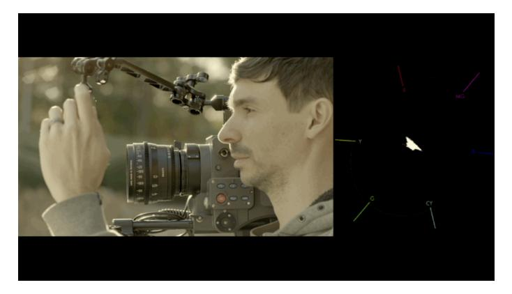
Though generally not considered as 'mission critical' during shooting as exposure scopes such as Waveform & Histogram, the **Vectorscope** plots the **chromaticity**, or the **hue + saturation** of your image onto a **color wheel** so you can help gauge **complimentary color**, ensure **skin tones** are being colorized properly, to visualize how overall scene color is being placed, and where potential adjustments may need to be made in general.
