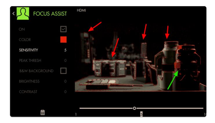
Notice how we are picking up many edges that are **not in focus** in addition to the areas that are in focus. **Increase** the next slider labeled 'Peak Thresh' to help eliminate the false positives.
