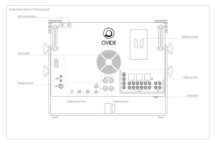
**Fan intakes:** This is the fan intake that blows air straight into the processor and GPU. Never block this airflow as it will permanently damage the unit and will void its warranty.
